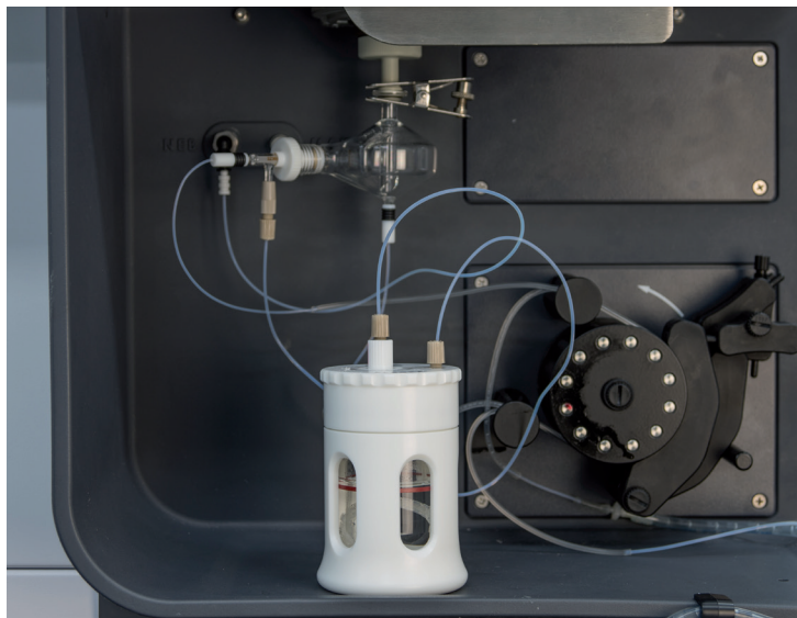
Figure 1. Glass Expansion High TDS Package for Agilent 5100 ICP-OES.
